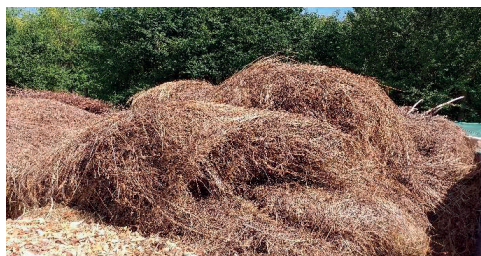
Figure 3. Straw waste used to produce bales, as the main structure for the multilayer biodegradable structures
