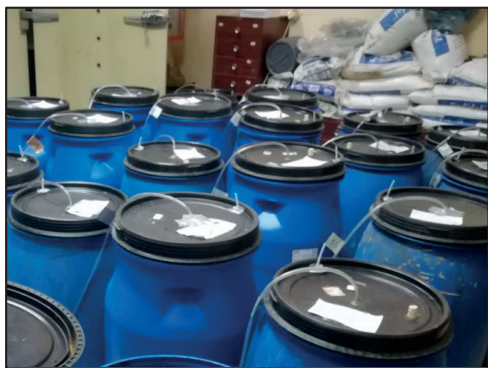
Figure 1. Apparatus setup for the greenhouse experiments on composting of solid fraction with different additives (control and Biochar). Each treatment and control have 3 replicates
