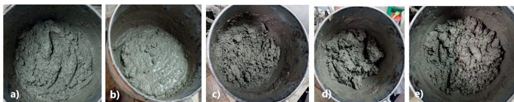
Figure 6. Fresh state aspect of the mortars: a) R1; b) R2; c) RS1-25%-0.56; d) RS1-25%-0.61; e) RS1-50%-0.61
