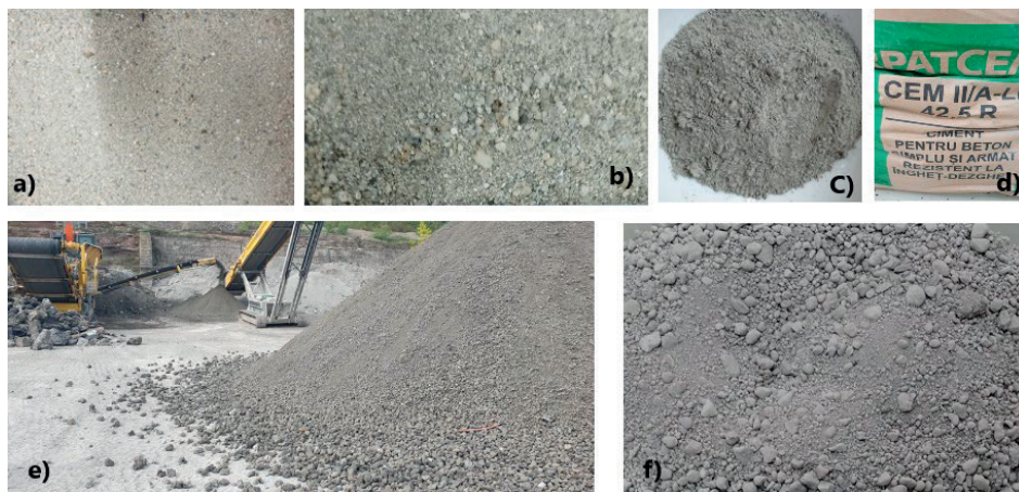
Figure 2. Raw materials for cement-based mortar mix design: a) and b) Natural sand 0/4 (S 0/4); c) and d) Binder - Carpatcement Portland Cement CEM II/A-LL 42.5 R; e) AdT: EOF (RS) derived from the aggregate crushing line, Caraş-Severin County; f) selected AdT: RS1
