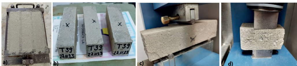
Figure 8. Hardened state characteristics of the mortars: a) and b) specimens' production; c) flexural strength determination by 3PB; d) compressive strength determination on halve-prism specimens
