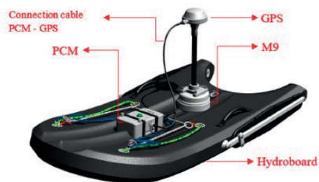
Figure 3. The M9 ADCP principal components
