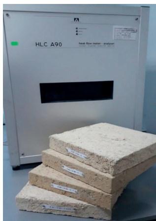
Figure 5. Testing thermal conductivity
