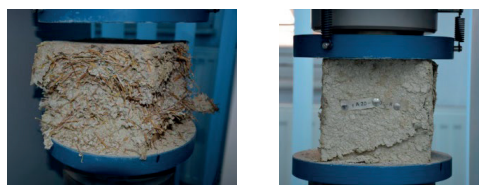
Figure 8. Testing compressive strength
