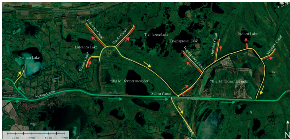
Figure 7. The assessment of the sediment (dis)connectivity in the study area (the main stream in green, in yellow the former meanders and the lateral canals, occasionally disconnected for the main stream at very low discharge and, in red the areas disconnected when the lateral connectivity is lost)
