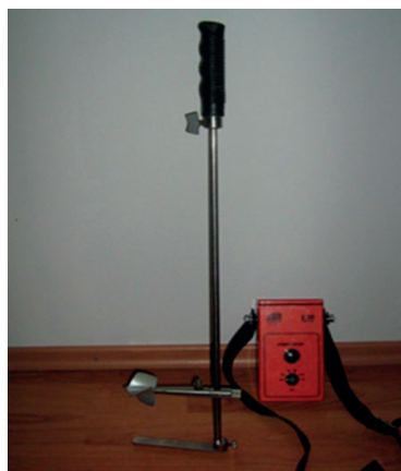
Figure 4. OTT type of hydrometric micro mill
