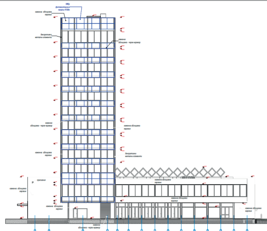
Figure 5. Layout of BIPV panels - west façade
