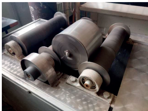
Figure 4. Rotary drum mill used in the printed circuit board grinding process
