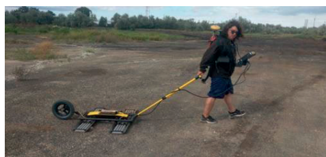
Figure 6. Georadar acquisition data with 100MHz antenna
