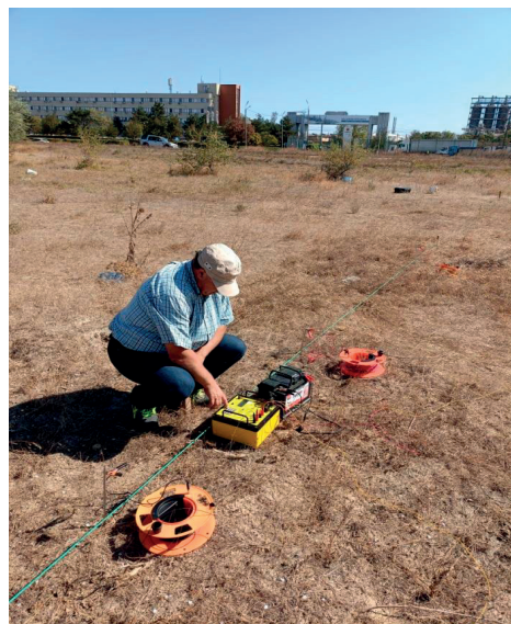
Figure 2. Geoelectric data acquisition using Ministing system from AGI
