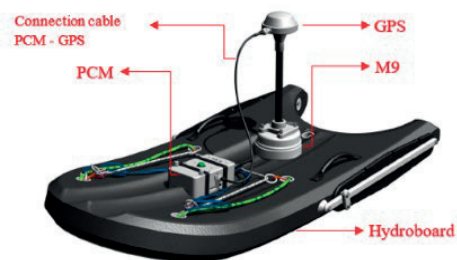
Figure 3. The M9 ADCP principal components
