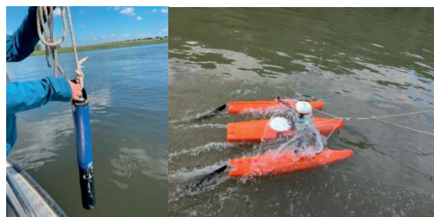
Figure 3. Multiparameter instrument model EX02 (left); ADCP River Ray 600 kHz (right)
