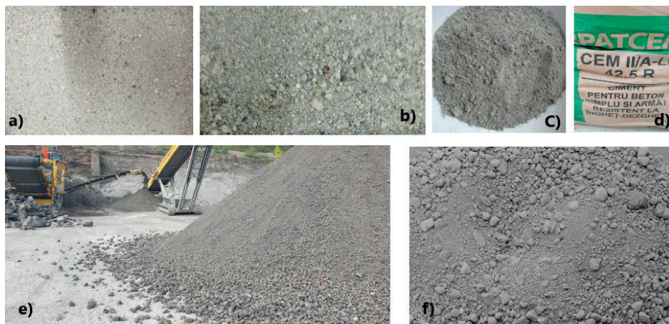
Figure 2. Raw materials for cement-based mortar mix design: a) and b) Natural sand 0/4 (S 0/4); c) and d) Binder - Carpatcement Portland Cement CEM II/A-LL 42.5 R; e) AdT: EOF (RS) derived from the aggregate crushing line, Caraş-Severin County; f) selected AdT: RS1
