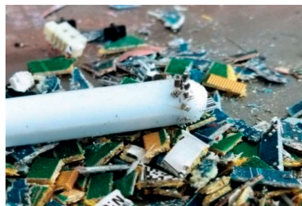
Figure 3. Separation of the ferrous metal fraction from the non-ferrous metal fraction
