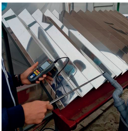
Figure 3. Measurement of the speed of the air current at the exit of the terminal tubes, with the Anemometer CIH20DL
