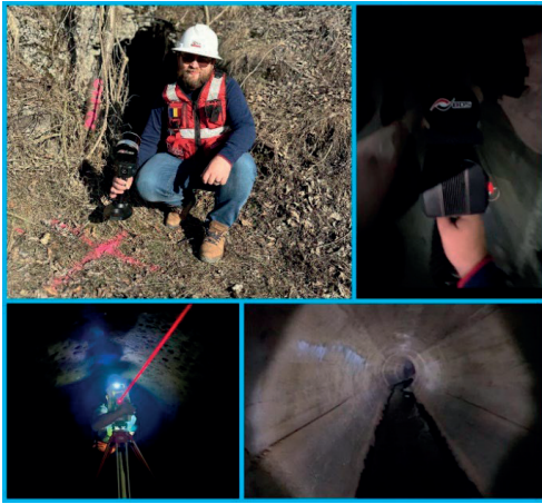
Figure 4. SLAM and TS mapping; video inspection
