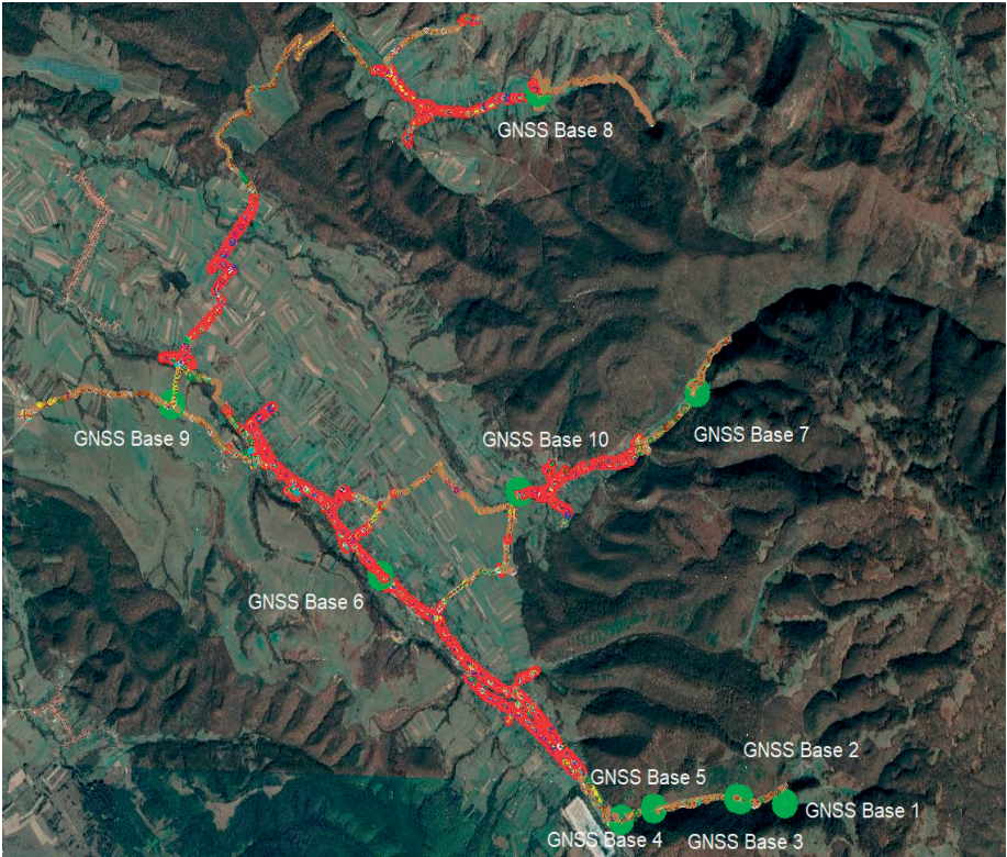
Figure 6. The location of the ten GNSS bases on the orthophoto plane, which were positioned in stage I, and were used as density points for the following stages of work
