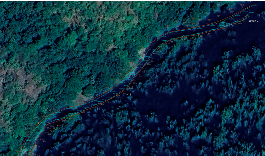
Figure 7. Overlay of the detailed plan of the water supply network on the orthophoto plane, in the spring 2 area
