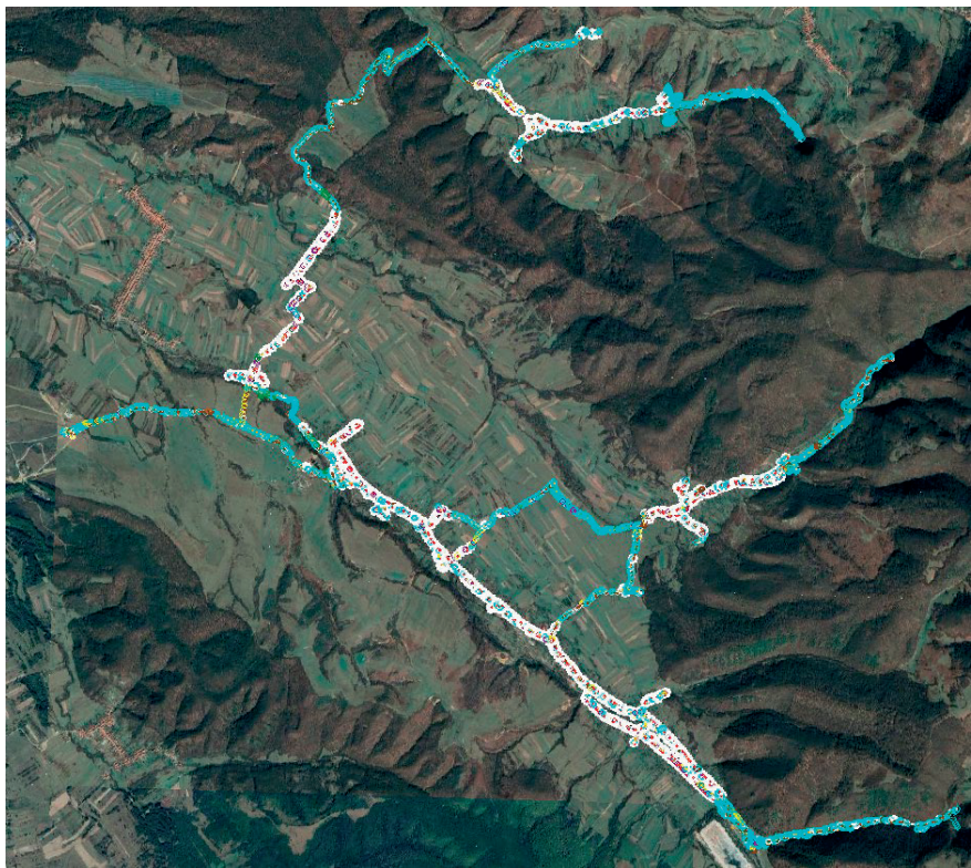
Figure 8. Detailed plan of the water supply and sewage network, superimposed on the orthophoto plane
