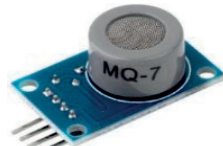
Figure 4. MQ-7 sensor module used for gas concentration monitoring (MQ7, 2025)
