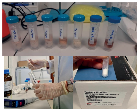
Figure 3. QuEChERS extraction steps
