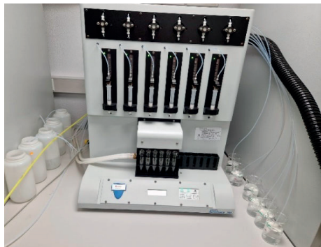
Figure 2. Automated solid phase extraction system
