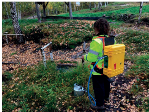
Figure 4. Soil flux survey conducted with West Systems portable fluxmeter in October 2022
