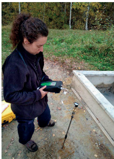
Figure 7. Soil gas survey using Gas Systems portable gas analyser and Durridge hardened steel probe next to a wet mofette (SG 11) in October 2022
