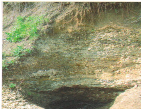
Figure 6. Hydrocarbon contamination of the geological formation located above the water table, due to seasonal variations
