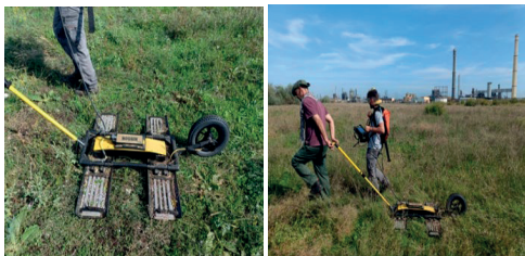
Figure 3. Data acquisition using GPR NOGIN
