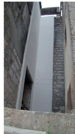
Figure 3. Test stand with ETICS prepared for fire resistance testing generated from the fire compartment
