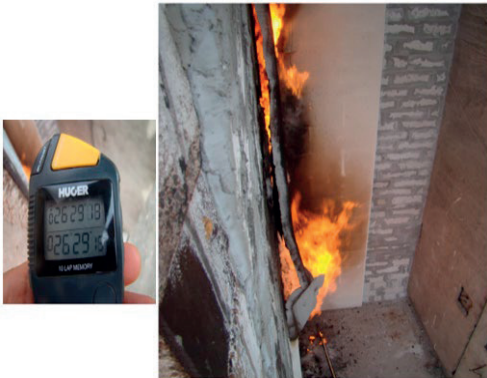
Figure 8. The beginning of the fire propagation on the height of the ETICS on the side wall
