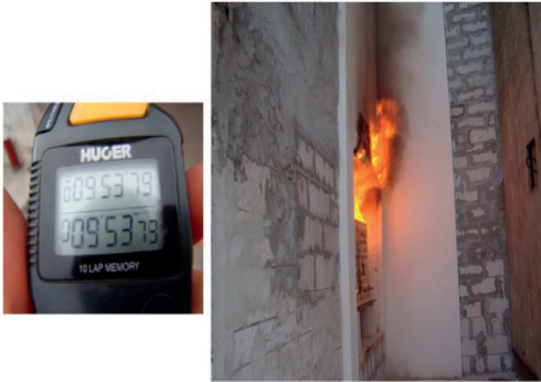
Figure 7. The beginning of the fire propagation on the height of the ETICS on the front wall
