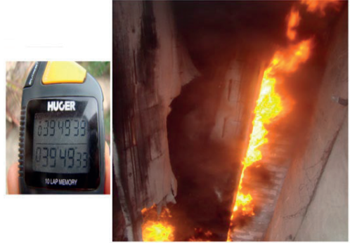
Figure 9. Complete combustion of the ETICS on the side wall to the fire compartment
