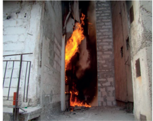
Figure 10. Burning particles detached from the thermal system
