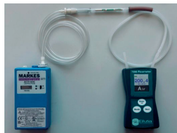
Figure 7. Flow Rate adjustment and flow monitoring
