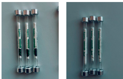
Figure 2. Tenax TA/Carboxen1018 and Tenax TA tubes
