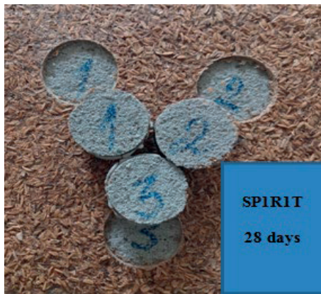
Figure 6. Appearance of the SP1R1T coating, containing rice husks and hemp fibers, and the way it breaks when pulled off, for determining adhesion at 28 days
