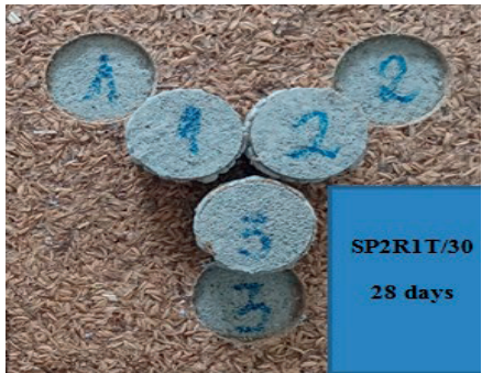
Figure 7. Appearance of the SP2R1T/30 coating, containing rice husks and hemp fibers, and the way it breaks when pulled off, for determining adhesion at 28 days
