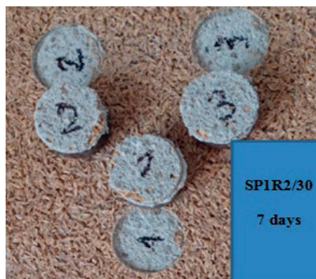
Figure 3. Appearance of the SP1R2/30 coating containing rice husks and the way it breaks when pulled off, for determining adhesion at 7 days
