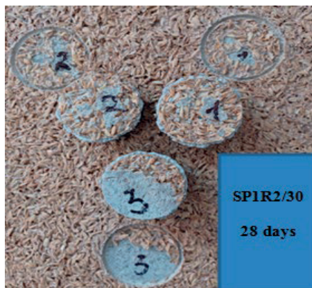
Figure 4. Appearance of the SP1R2/30 coating containing rice husks and the way it breaks when pulled off, for determining adhesion at 28 days
