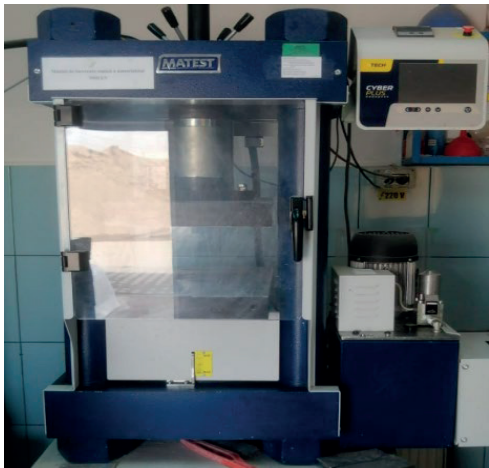
Figure 3. Matest 2000KN concrete press
