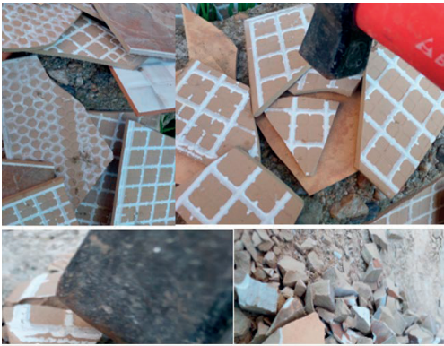
Figure 5. The grinding process of ceramic waste
