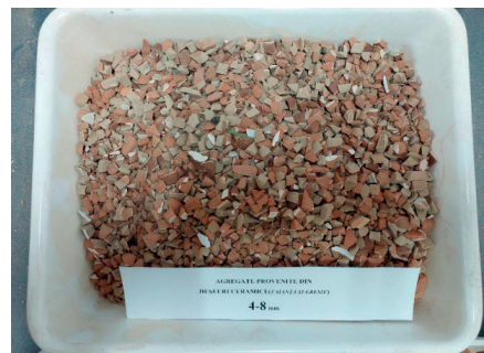
Figure 2. Aggregates from ceramic waste size 4-8 mm
