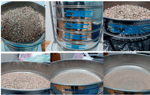
Figure 6. Size sorting of shredded ceramic waste
