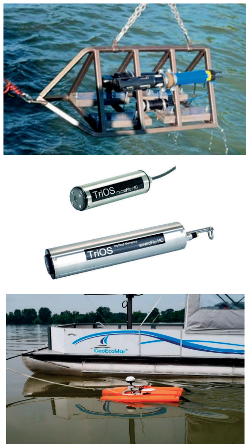
Figure 2. Multiparameter probe, model EX02 and the PAH probes, microFlu from Aquam and ADCP River Ray 600 kHz
