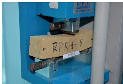
Figure 7. The mode of failure of the sample subjected to bending
