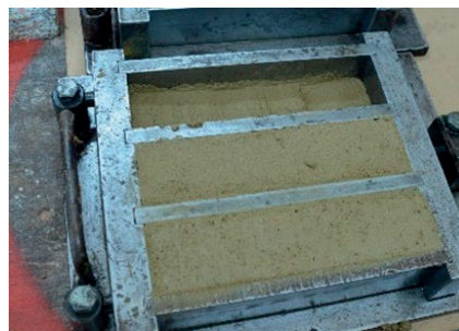
Figure 3. Casting fresh clay mixture in metal moulds
