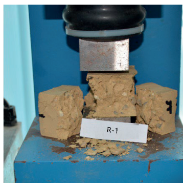
Figure 8. Compressive strength of the prism halves
