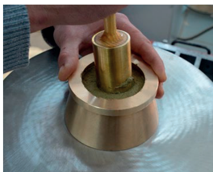
Figure 2. Determination of the consistency of the fresh clay mixture
