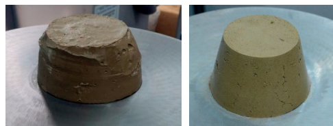
Figure 4. Different consistency of the fresh clay mixture
