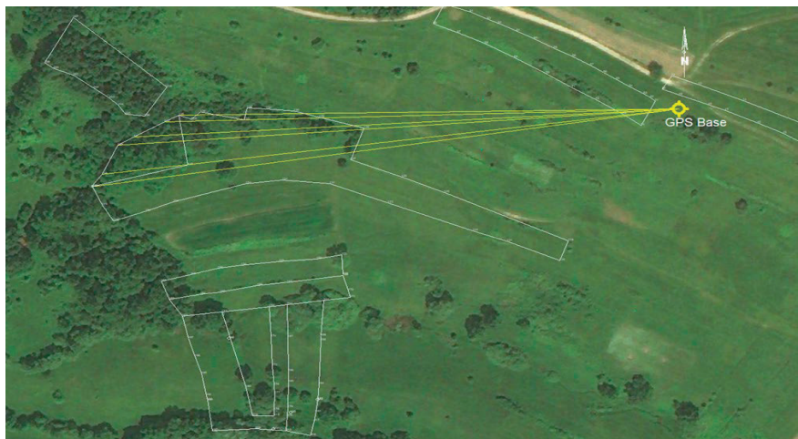
Figure 6. Positioning of plots occupied by forest vegetation using the RTK method, with radio modules
