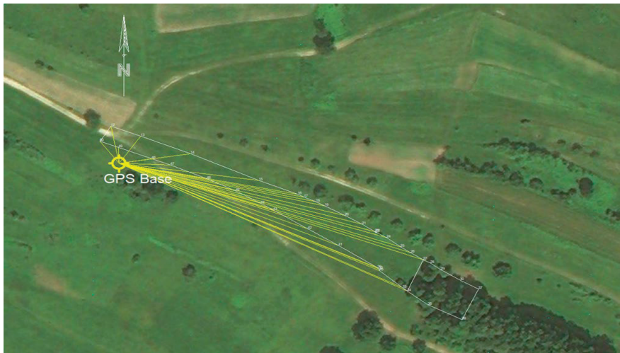
Figure 7. Positioning of characteristic points of parcels by RTK method with internal radio - external radio modules
