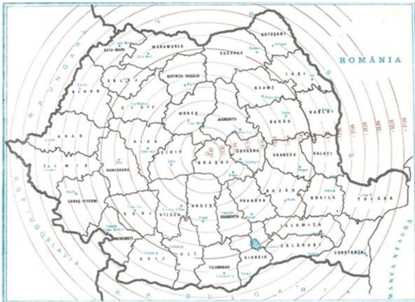
Figure 1. Distance deformations in Stereographic 1970 (Iosif Gh., 2012)
