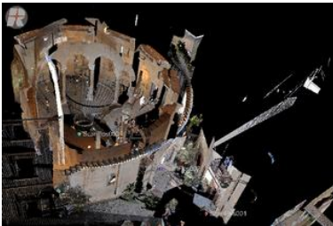
Figure 9 A rendering of photographic pictures over the 3D LASER Scanning Surveying of the Tempio di San Giovanni al Sepolcro, in Brindisi, Italy
