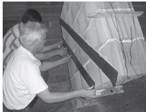
Fig. 14. Making specimens, by applying the Carבודur S 1012 strips
